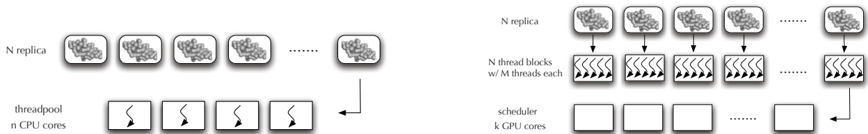
Figure 2: Schematic representation of multithreaded parallelization on CPUs on the left and twofold parallelization on GPUs on the right.
